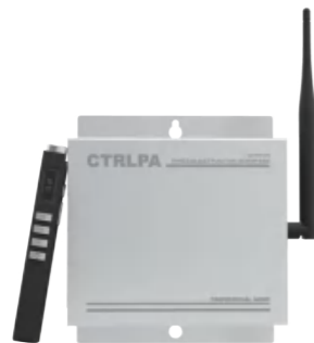
CT/HY170 2.4G 数字无线语音模块 Digital Wireless Voice Module
